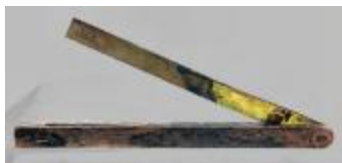
Tool, Shipbuilding- Try Square For Angle Measure (90.58)
